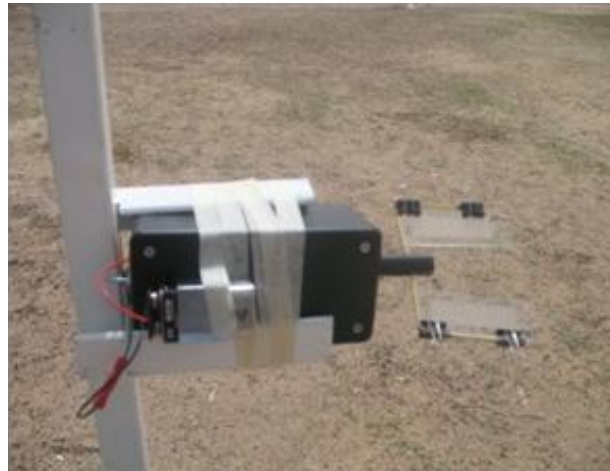
Figure 6.2-1. Rotoslide sampler as attached to sampling pole.
